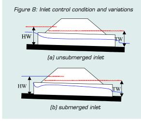
This happens when the slope of the culvert is steeper than the critical slope. When the conduit flows with an unsubmerged inlet, the flow passes through critical depth at the entrance to the culvert. When the culvert flows with a submerged inlet, which will occur when HW/D > 1.5, the inlet will act as an orifice and the flow will contracted as if flowing through a sluice gate.
