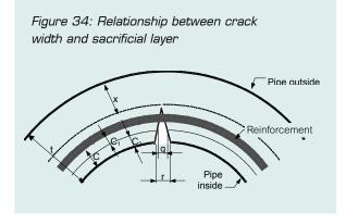
Example: If a 900 mm diameter concrete pipe with a standard wall thickness of 93 mm has a sacrificial layer of 20 mm, what is the allowable crack width at proof load? Standard cover to steel is 10 mm.
