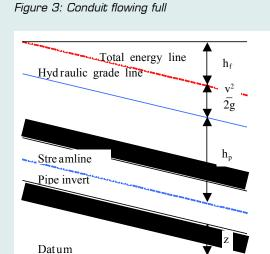
The total energy at any point along a conduit operating under pressure can be defined by Bernoulli's equation:
