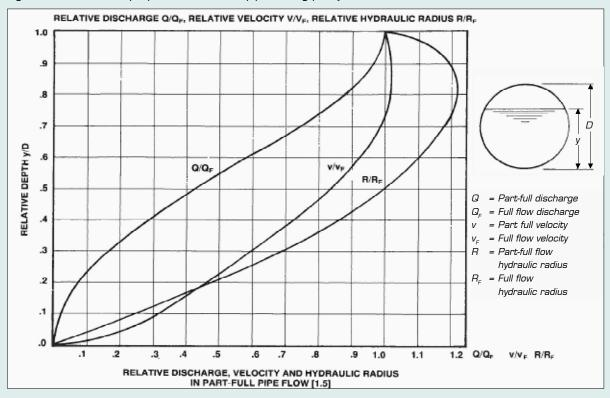
Figure 6: Relative flow properties of circular pipe flowing partly full
