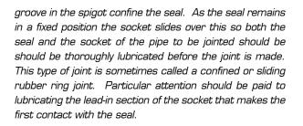
The advantage of this type of joint is that the outside diameter of the pipe remains constant making the pipe ideally suited for jacking. For jacking pipes from 900 mm in diameter and larger use this joint type. However for sewers this type of joint is seldom used for pipes of less than 1500 mm in diameter. Most pipes larger than 1800 mm in diameter are made with this type of joint.
