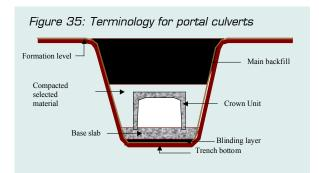
As portal culverts are rectangular two dimensions determine their size. Hence, the relationship between the load to be carried and the required strength cannot be simplified as it can with pipes. Hence, the strength required is determined by using a direct approach. The procedure adopted is:
