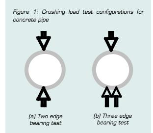
The three edge-bearing test is preferred as the pipe is firmly held in place by the bottom two bearers before and during the test. With the twoedge bearing test there is the danger that the pipe could slip out of the testing apparatus or might not be perfectly square when tested.
