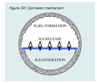
The most important factors contributing to  $H_2S$  generation in the effluent are:
