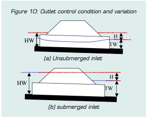
The water surface will not pass through critical depth at any section of the culvert hence there are no sections where there is a fixed depth discharge relationship. The major energy loss will be at the outlet.
