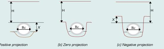
Example 1. Determination of backfill load under the following conditions: Embankment installation, positive projection. Pipe D = 525 mm; Projection ratio: x/D = 0.7; Foundation material: rock (r<sub>s</sub> = 1); Density of fill: 1 750 kg/ m<sup>3</sup>; Height of fill above top of pipe: 3.5 m.
