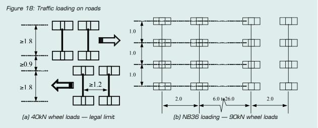
For the NB loading, 1 unit = 2.5 kN per wheel = 10 kN per axle and = 40 kN per vehicle. For the NB36 vehicle = 90 kN per wheel = 360 kN per axle.
