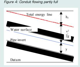
The total energy at any point along a conduit flowing partly full can be defined by the energy equation:
