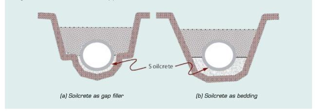
Soilcrete consists of a granular material that has between 3% and 6% of cement added to it and is made as a flowable mix with a slump of >200mm. There should be no organic material in the soil used and ideally the clay content should be minimal. The soilcrete is stronger that soil, having a strength between 0.5 and 1.0 MPa. This material can be used in two ways, namely as a gap filler or as a bedding as illustrated in Figures 29 (a) and (b).
