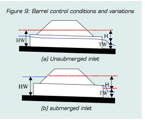
Outlet control occurs when the water level downstream of the culvert controls the volume of water that can flow through the culvert by drowning out either inlet or barrel control conditions. In other words when the capacity of the barrel or the inlet cannot be realised because there is no free discharge downstream of the culvert.
