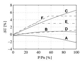
Fig. 8. Voltage level influence by different WECS. A-C Fixedspeed system, D-F variable-speed system. A & D: X/R=5, B: X/R=2, C: X/R=1.1, E: X/R=1.1 over voltage limit 3% and, F: X/R=1.1 over voltage limit 5%.
