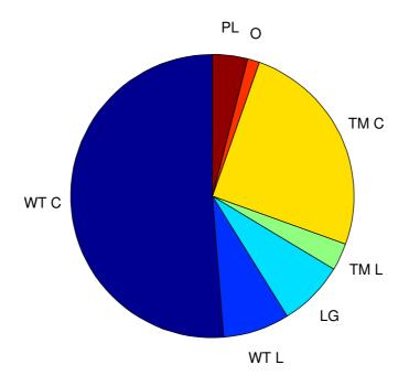
Figure 5.10: The energy production cost divided into components for the large AC wind farm for the reference case.
