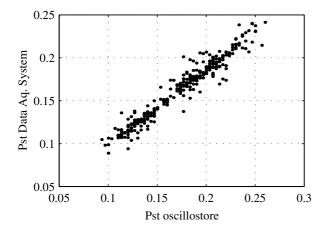
Fig. 3.  $P_{st}$  level on the local 400 V grid determined using Oscillostore and from data aquisition system, during three hours of operation with low flicker levels. One minute  $P_{st}$  values.
