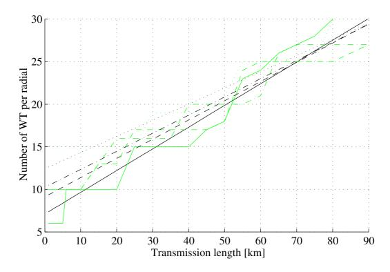
Figure 5.15: Number of wind turbines per radial for 40kV transmission voltage. Black theoretical curve and grey actual curve. Solid 60MW park, dashed 100MW, dash-dotted 160MW and dotted 300MW wind park.
