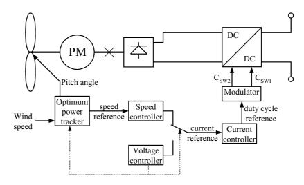
Figure 6.2: The layout of the control system for the series connected wind turbine.
