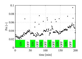
Fig. 5.  $P_{st}$  contribution (flicker emission) from turbine four with the other wind turbines on (gray patch intervals) and off. One minute  $P_{st}$  values.
