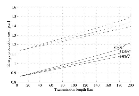
Figure 5.17: The normalized energy production cost for the different configurations of the large DC system. For a 300MW wind park, an average wind sped of 10m/s and for different transmissions lengths.
