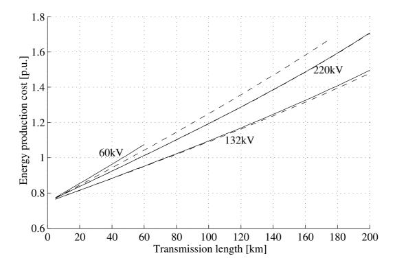
Figure 5.9: The normalized energy production cost for the different configurations of the large AC system. For a 100MW wind park, an average wind sped of 10m/s and for different transmissions lengths. Solid fix speed wind turbines and dashed wind turbines with the DFIG system.
