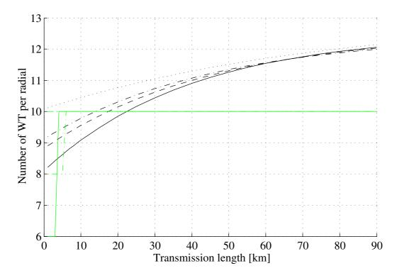
Figure 5.5: Number of wind turbines per radial for 22kV transmission voltage. Black theoretical curves and grey actual curves. Solid 60MW park, dashed 100MW, dash-dotted 160MW and dotted 300MW wind park.
