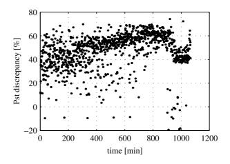
Fig. 13. Discrepancy between the actual flicker emission and the formula from IEC-61400-21, 70 degrees grid impedance angle.
