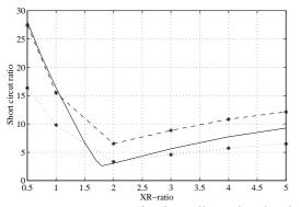
Figure 7. Limiting curves for the stall-regulated turbines. The solid curve is for the 2.5 % static voltage level change limit, the dashed curve is for flicker contribution of 0.25 with one turbine and the dotted curve is for flicker contribution of 0.25 with a wind farm consisting of 3 wind turbines.
