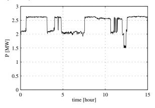
Fig. 11. Active power from Bockstigen during a high wind speed and high load condition.
