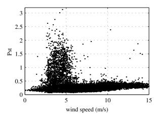
Fig. 14.  $P_{st}$  contribution as function of wind speed at Alsvik. One minute  $P_{st}$  values.
