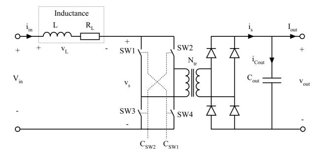
Figure 6.3: The scheme of the full bridge isolated boost converter that is used for derivation of the current controller.
