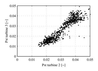
Fig. 11. Flicker emission from the no-loaded generator compared to flicker emission from turbine 3, 70 degrees grid angle. One minute  $P_{st}$  values.
