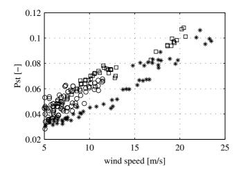
Fig. 7.  $P_{st}$  contribution as function of wind speed, X/R=1, legend as in Fig 6.
