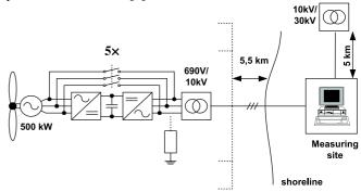
Figure 2. The electrical system of the Bockstigen wind park.
