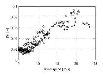
Fig. 9.  $P_{st}$  contribution as function of wind speed, X/R=5, legend as in Fig 6.
