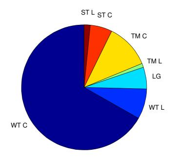
Figure 5.21: The energy production cost divided into components for the series DC wind farm for the reference case.
