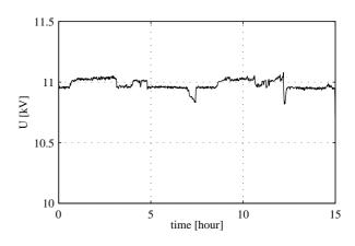
*Fig. 12. Voltage level at Bockstigen during a high wind speed and high load condition.*
