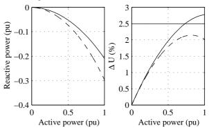
Figure 5. Reactive power consumption for two different induction generators, X/R=1.7.
