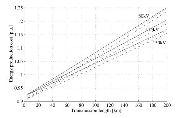
Figure 5.12: The normalized energy production cost for the different configurations of the AC/DC system. For a 300MW wind park, an average wind sped of 10m/s and for different transmissions lengths. Solid fix speed wind turbines, dashed wind turbines with the DFIG system and dotted fix speed wind turbines speed controlled with the offshore converter station.
