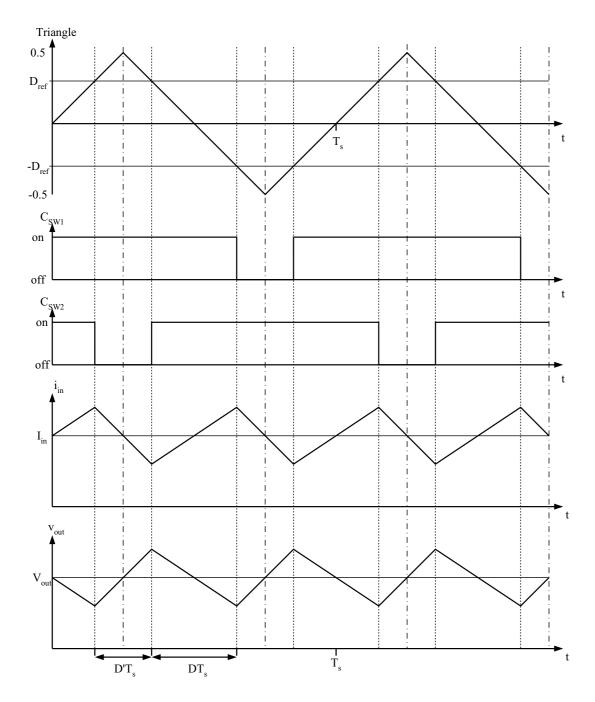
Figure 6.4: Triangle modulation to obtain the on and off times for the switches, and corresponding current and voltage waveforms.
