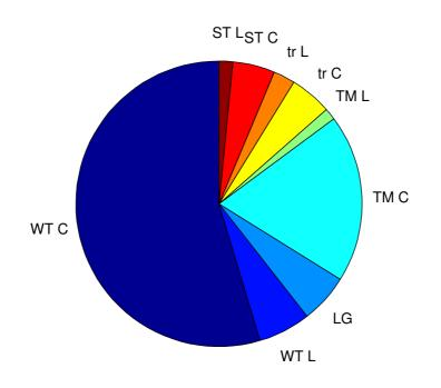
Figure 5.16: The energy production cost divided into components for the small DC wind farm for the reference case.
