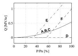
Fig. 9. Reactive power demand of different WECS. Notation as in Fig. 8.
