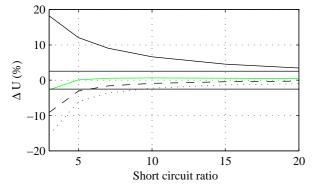
Figure 4. Steady-state voltage as function of short circuit ratio for different XR-ratios. Lines as in Fig. 3.
