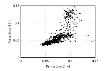
Fig. 12. Flicker emission from the no-loaded generator compared to flicker emission from turbine 3, 30 degrees grid angle. One minute  $P_{st}$  values.
