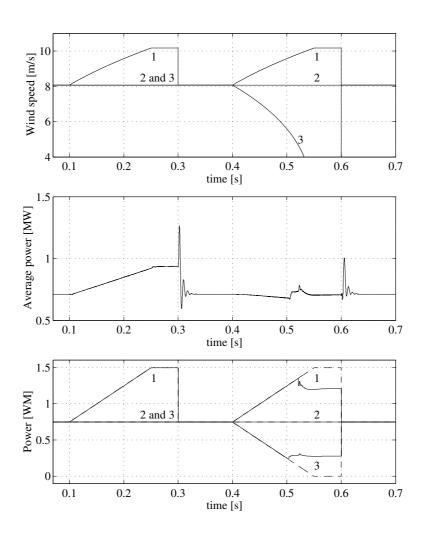
Figure 6.10: The input to the simulations of the three series connected converters, the different inputs to the three wind turbines are numerated 1 to 3. In the top plot the wind speeds for the wind turbines are shown. In the middle plot the average output power and in the bottom plot the optimal turbine power (black dashed lines), actual turbine power (solid black line) are shown.
