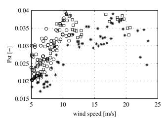
Fig. 8.  $P_{st}$  contribution as function of wind speed, X/R=2, legend as in Fig 6.
