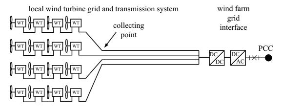
Figure 2.5: The electrical system for the small DC wind park.
