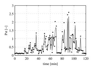
Fig. 4.  $P_{st}$  level on the local 400 V grid determined using Siemens Oscillostore P513 (dots) and from data acquisition system (solid line), operation at high flicker levels.
