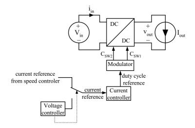
Figure 6.5: The test scheme for evaluation of the performance of one full bridge isolated boost converter.
