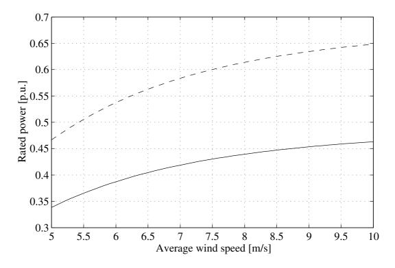
Figure 5.11: Rated power of the HVDC-station in p.u. of the rated power of the wind park as function of the average wind speed for different investment factors. Solid  $B_I = 12$  and dashed  $B_I = 24$ .
