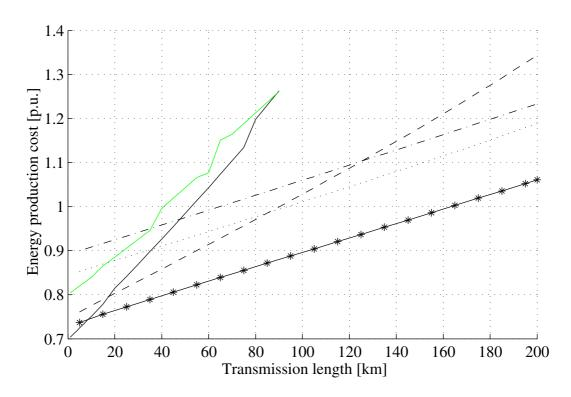
Figure 5.2: The normalized energy production cost of the different 160MW wind parks as function of the transmission distance and at a average wind speed of 10m/s. Solid small AC, dashed large AC, dash-dotted AC/DC, grey small DC, dotted large DC and solid with stars series DC.
