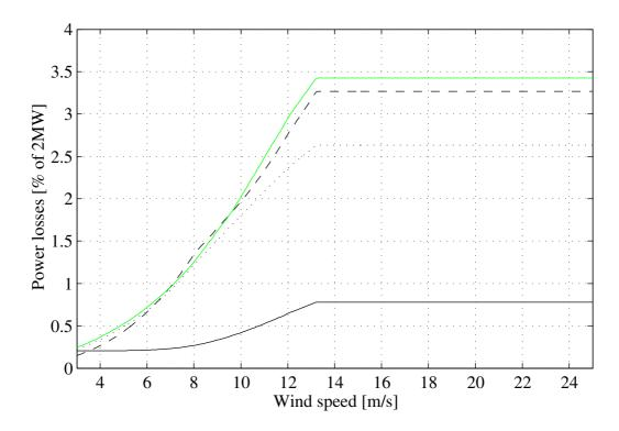
Figure 4.7: The losses of the 2MW full variable speed turbine equipped with a asynchronous generator. Solid transformer losses, dashed generator losses, dotted gearbox losses and grey converter losses.
