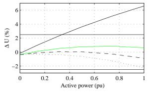
Figure 3. Voltage change as a function of produced power for various X/R-ratios. The grid strength is 10 times the rating of the turbine. Solid XR=0.5, Grey XR=2, Dashed XR=3, Dotted XR=5. The 2.5 % limits are marked with solid lines.
