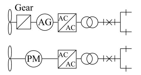
Figure 4.6: Principal schemes of the 2MW full variable speed turbine, top with asynchronous generator and bottom with permanently magnetized generator.
