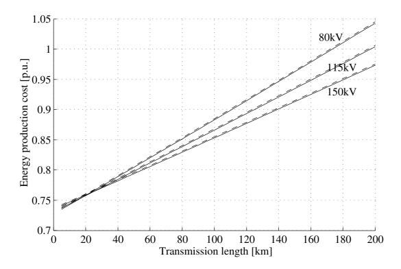
Figure 5.20: The normalized energy production cost for the different configurations of the series DC system. For a 300MW wind park, an average wind sped of 10m/s and for different transmissions lengths. Solid maximum 4 failed wind turbines per leg, dashed maximum 8 failed wind turbines per leg.
