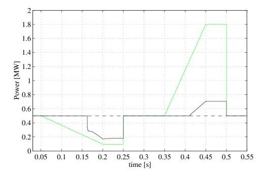
Figure 6.7: The grey line shows the average power production of the wind turbines in the leg, the black solid line shows the actual output power of the investigated wind turbine and the black dashed line shows the desired turbine output power.
