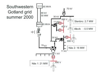
Fig. 2. Schematic sketch of the Näsudden grid.
