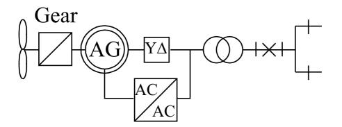
Figure 4.4: Principal scheme of the 2MW semi variable speed wind turbine.
