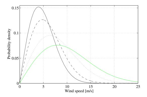
Figure 3.1: Rayleigh distribution function for different mean wind speeds, solid 5m/s, dashed 6m/s, dotted 8m/s and grey 10m/s.
