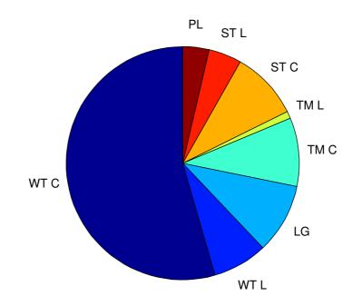
Figure 5.13: The energy production cost divided into components for the AC/DC wind farm for the reference case.
