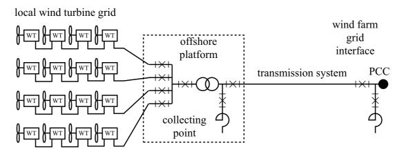
Figure 2.3: The electrical system for the large AC wind park.
