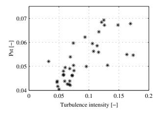
Fig. 10.  $P_{st}$  contribution as function of turbulence intensity, for wind speeds between 12 and 13 m/s. X/R=1, one minute  $P_{st}$  values.
