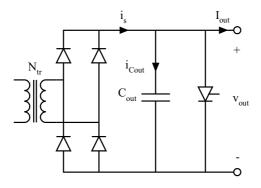
Figure 6.12: Protection for the series connected wind turbine.
