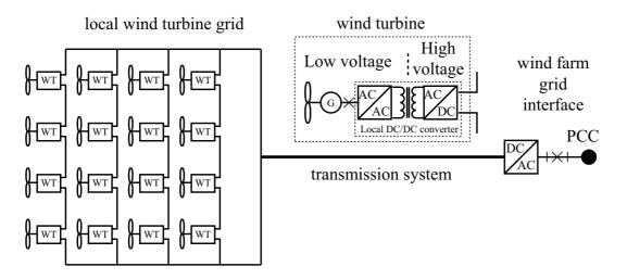
Figure 2.7: DC electrical system with series connected wind turbines.
