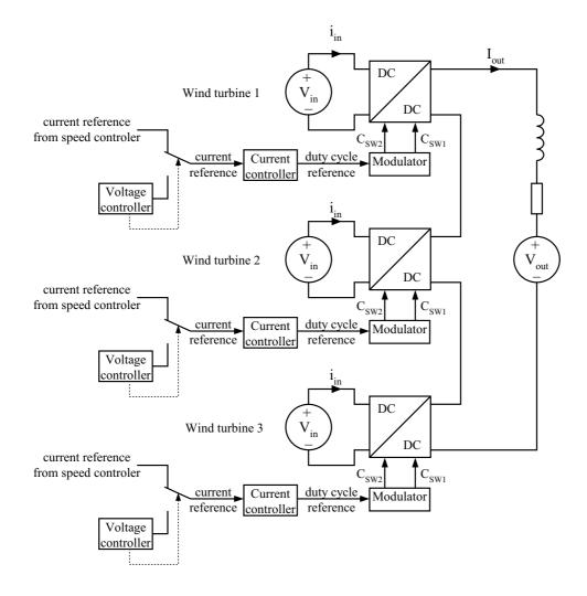
Figure 6.9: The test scheme for evaluation of the performance of three series connected full bridge isolated boost converter.
