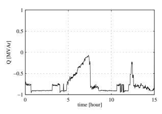
*Fig. 13. Reactive power from Bockstigen during a high wind speed and high load condition.*
