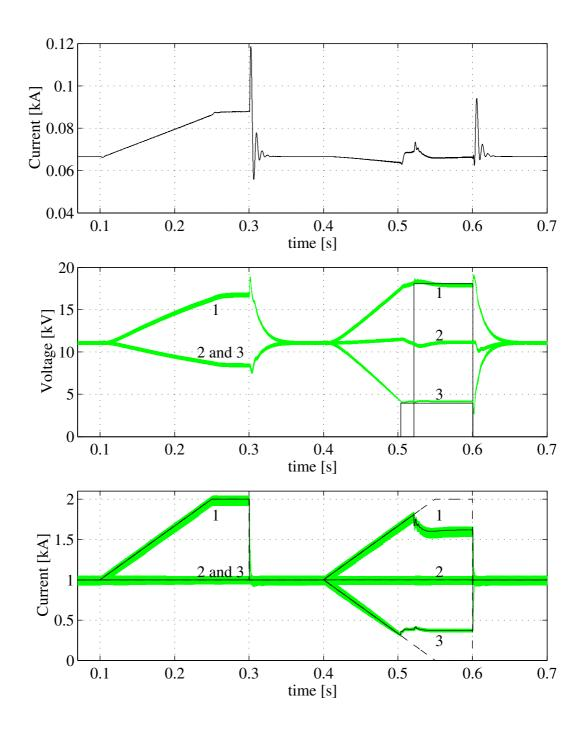
Figure 6.11: The results from simulations of the three series connected converters, the results are numerated 1 to 3 for the different converters. In the top plot the current that goes through the leg,  $I_{out}$ , is shown. In the middle plot the output voltage for the three converters are shown and in the bottom plot the input current (grey lines), input current reference (solid black line) and the input current reference from the speed regulator (dashed black lines) are shown.
