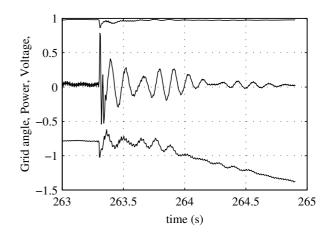
Fig. 15. Voltage (pu, upper line) and grid angle (no relevant scale, lower line) dip causing a power oscillation (pu, medium line).
