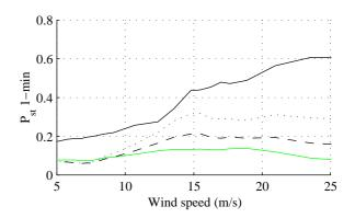
Figure 6. One minute flicker value and for the fixed-speed stall-regulated turbine using different XR-ratios. Short circuit ratio is equal to 10. Lines as in Fig. 3.
