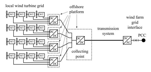
Figure 2.6: The electrical system for the large DC wind park with two DC transformer steps.
