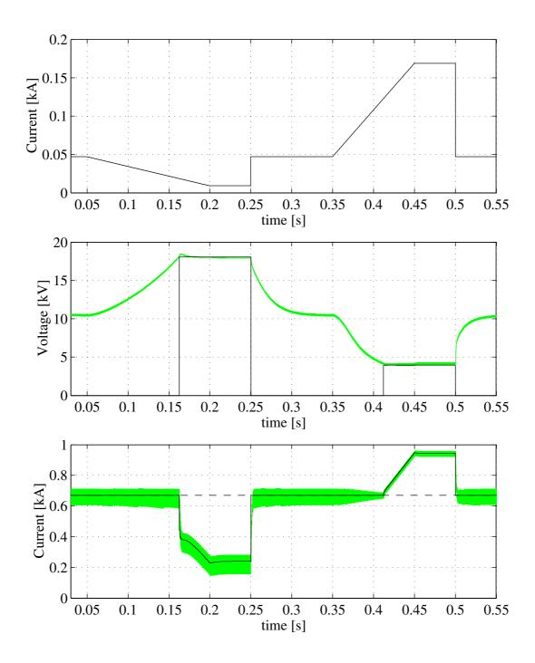
Figure 6.8: The currents and voltages of the investigated wind turbine. In the top plot the output current is shown. In the middle plot the output voltage (grey line) and the output voltage reference (black line) when the output voltage regulator is active are shown. In the bottom plot the input current reference (black solid line), the input current (grey line) and the input current reference from the speed regulator (black dashed line) are shown.
