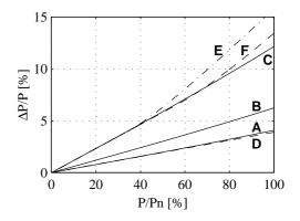
*Fig. 10 - Supply line losses by different WECS. Notation as in Fig. 8.*
