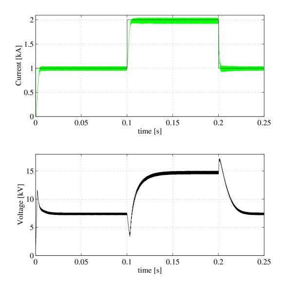
Figure 6.6: In the top plot the input current reference, black line, and the input current, grey line, are shown. In the bottom plot the output voltage is shown.
