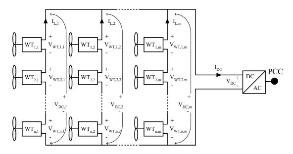
Figure 6.1: The layout of the series connected wind park.
