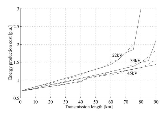
Figure 5.7: The normalized energy production cost for the different configurations of the small AC system. For a 60MW wind park, an average wind sped of 10m/s and for different transmissions lengths. Solid with fix speed wind turbines and dashed wind turbines with the DFIG system.
