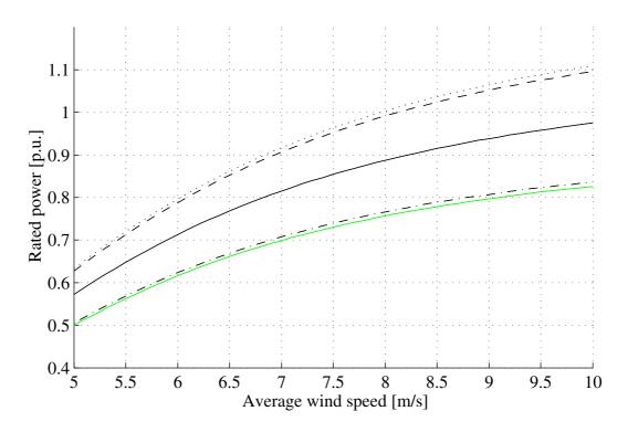
Figure 5.4: Rated power of the transformer in p.u. of the rated power of the wind park as function of the average wind speed for different rated powers of the wind park and different investment factors. Solid 150MW  $B_I = 19$ , dash-dotted 60MW  $B_I = 19$ , dotted 300MW  $B_I = 19$ , grey 150MW  $B_I = 14$  and dashed 150MW  $B_I = 24$ .
