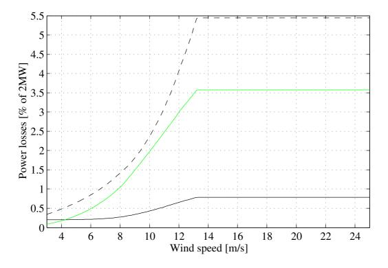
Figure 4.8: The losses of the 2MW full variable speed turbine equipped with a permanent magnetized generator. Solid transformer losses, dashed generator losses and grey converter losses.
