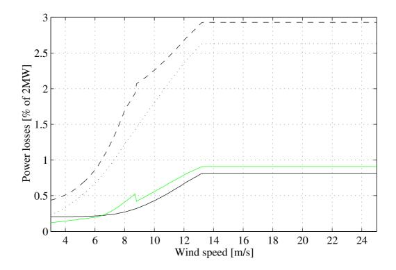
Figure 4.5: The losses of the 2MW semi variable speed wind turbine. Solid transformer losses, dashed generator losses, dotted gearbox losses and grey converter losses.
