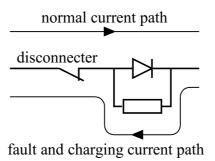
Figure 6.14: Scheme of the DC-breaker.
