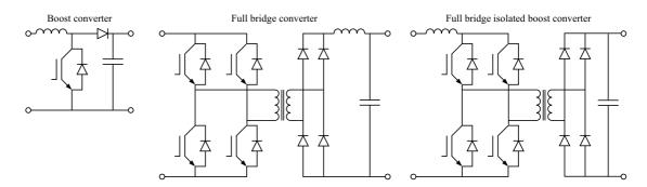
Figure 4.9: Principal scheme of the three most interesting DC/DC converter topologies.
