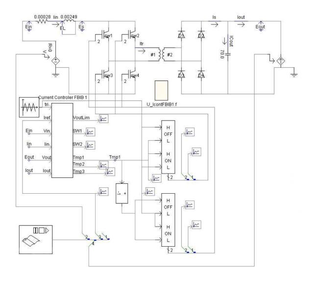
Figure B.1: Printout over the full bridge isolated boost converter implemented in  $\rm EMTDC^{\textcircled{O}}$
