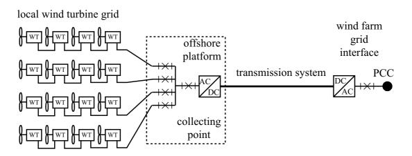
Figure 2.4: The electrical system for the AC/DC wind park.
