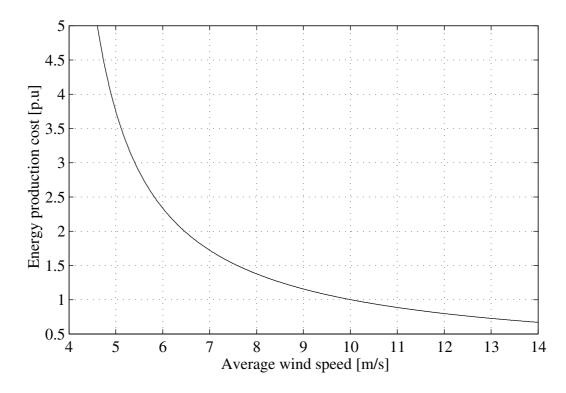
Figure 5.3: Energy production cost as function of the average wind speed, normalized with the prize at a average wind speed of 10m/s.
