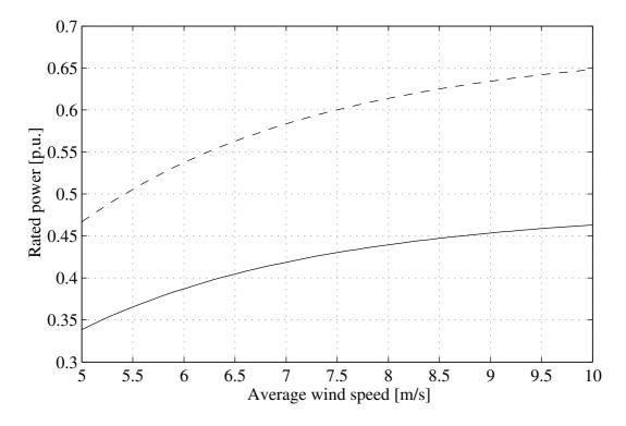
Figure 5.14: Rated power of the DC-transformer in p.u. of the rated power of the wind park as function of the average wind speed for different investment factors. Solid  $B_I = 12$  and dashed  $B_I = 24$ .
