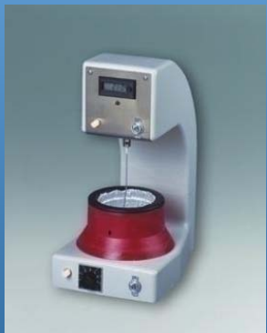
Gel Timer Measures the gel time of the resin
