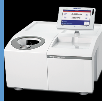
Differential Scanning Calorimeter Measures the Glass Transition temperature ( T_g )
