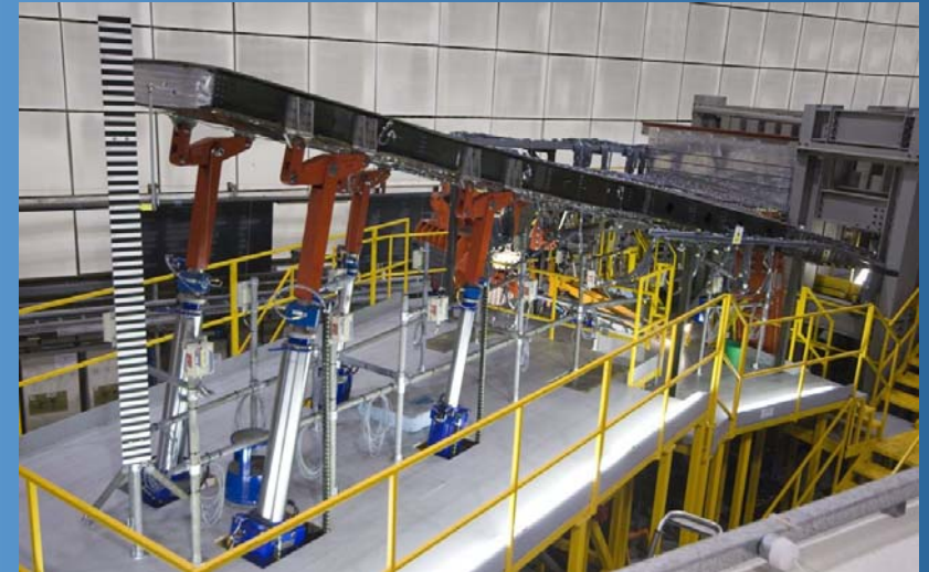
Fatigue Testing of F18 wing
