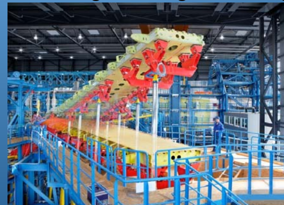
Fatigue Testing of F18 wing
