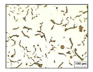
*Figure 8 – CGI typical microstructure: 5% nodularity, 9% graphite, 265 particles/mm<sup>2</sup>.*
