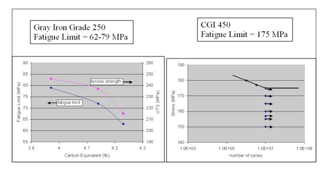
Figure 11 - Fatigue Limit results for an I6 cylinder block – 5.9 L – 150 kg. Samples from the main bearings, push-pull test (R = -1, 10 Hz). Gray Iron Grade 250, 100% pearlite, 210-250 HB, CrCuSn. CGI Grade 450. 2-4% nodularity, <2% ferrite. 230-255 HB. (Guesser, 2003).
