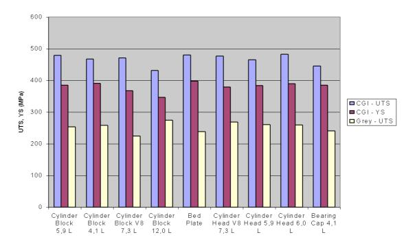
*Figure 9 - Mechanical properties of gray iron and CGI grades 400-450. 195-230 HB. Samples taken from the castings (Guesser, 2003).*
