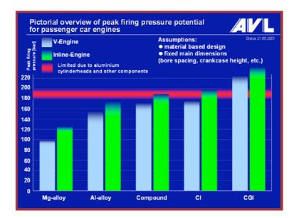
Figure 3 – Peak firing pressure limits for various materials in diesel engine cylinder block (Marquard & Sorger, 1997)
