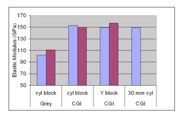
*Figure 10 – Elastic modulus of gray iron and CGI grade 400. 12.0L I6 cylinder block (Guesser, 2003).*
