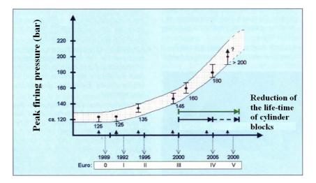
Figure 7 – In order to fulfill emissions standards requirements, the peak firing pressure in truck engines must surpass 200 bar, according to MAN (Vollrath, 2003).
