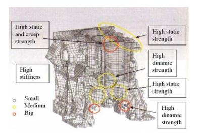
Figure 4 – The one-dimensional era of engine design is finished. The current approach considers the loads acting at each point of the engine block. (Vollrath, 2003)
