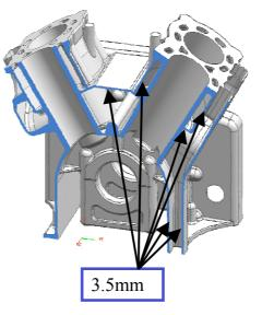
Figure 6 - Current wall thickness for Cyl. Blocks in CGI in production at Tupy Fundições.
