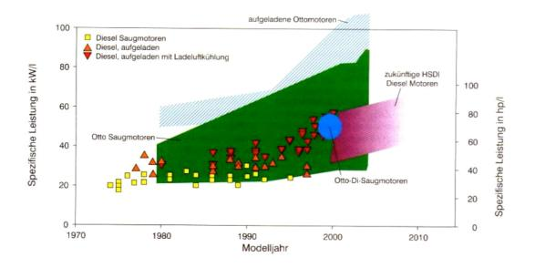
Figure 2 – Increase of the specific power of engines (FEV - Pischinger & Ecker, 2003)
