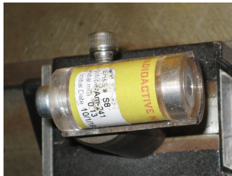
Figure 6: Am-241 Source in Place on its Holder
