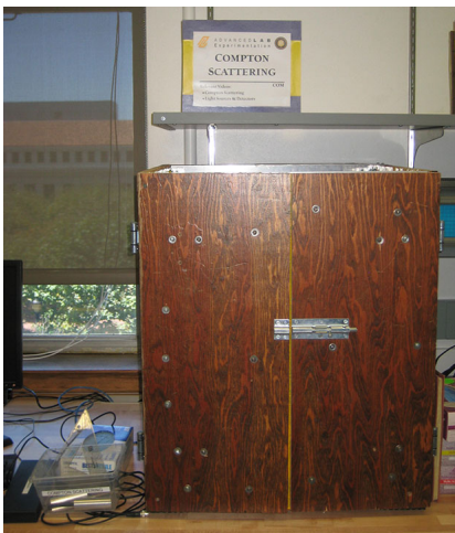
Figure 3: Lead-Shielded Box for the Compton Apparatus. Click here to see larger picture
