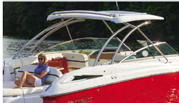
This top with an electrically deployable SureShade is standard equipment on model R35. A color-accented headliner is optional.
