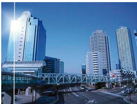
CCD shows smearing (vertical streaking) in very bright areas.
