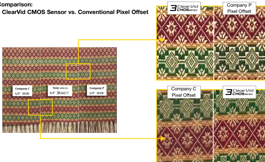
Interpolation processing on the 3 ClearVid CMOS Sensor is performed independently on each chip (R, G, and B), assuring maximum resolution regardless of the subject's color mix.
