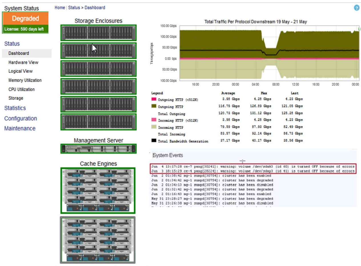
Figure 5-1 Failed Cache Engine
