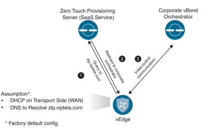
Figure 4-13 Zero Touch Provisioning Workflow
