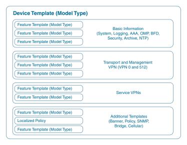
Figure 4-2 Device Template Structure
