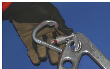
Twist carabiner so that gate opening is easily accessed
