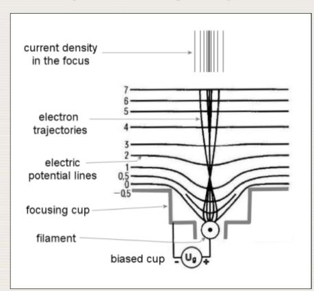
Numbers indicate potential difference near the cup in kV With an increasing negative bias voltage at the focusing cup the focus size will decrease and finally the electron current will be pinched **Off**
