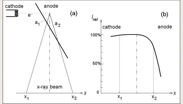
(a) Absorption of X rays at the cathode side of the X ray field
