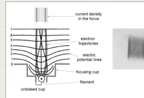
The typical **Bimodal** distribution of the current density can be seen in a pinhole image of the focus
