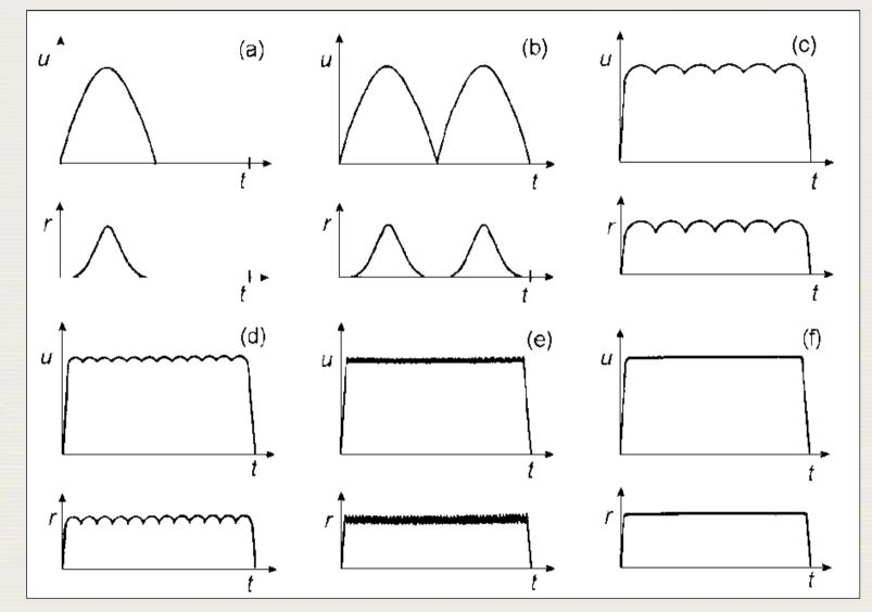
Voltage waveforms u and associated tube output (dose rate) r for (a) 1-pulse (b) 2-pulse (c) 6-pulse (d) 12-pulse (e) high-frequency (f) constant voltage generators
