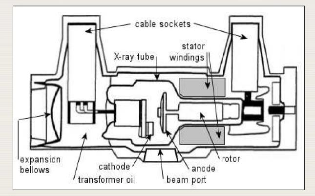
Typical housing assembly for a general purpose XRT
