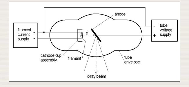
Principle components of an X ray tube are an **Electron Source** from a heated tungsten filament with a focusing cup serving as the tube **Cathode**, an **Anode** or **Target** and a **Tube Envelope** to maintain an interior vacuum
