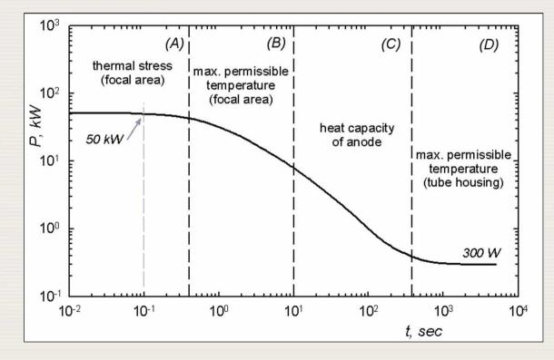
Maximum Permissible Tube Load vs. time for a single exposure, constant current, 100 kV tube voltage and a 50 kW tube
