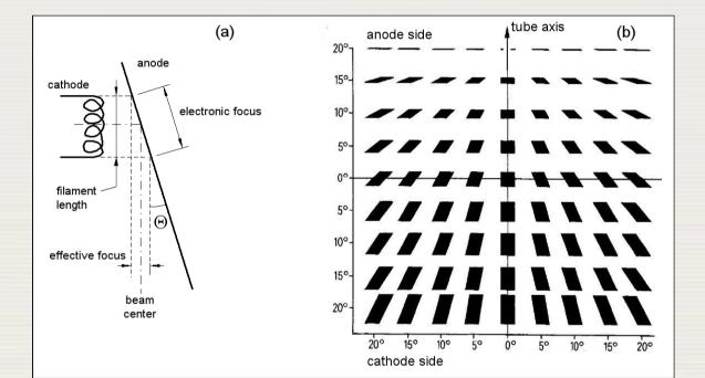
(a) **Line Focus Principle**: the length of the filament appears shortened in the beam direction
