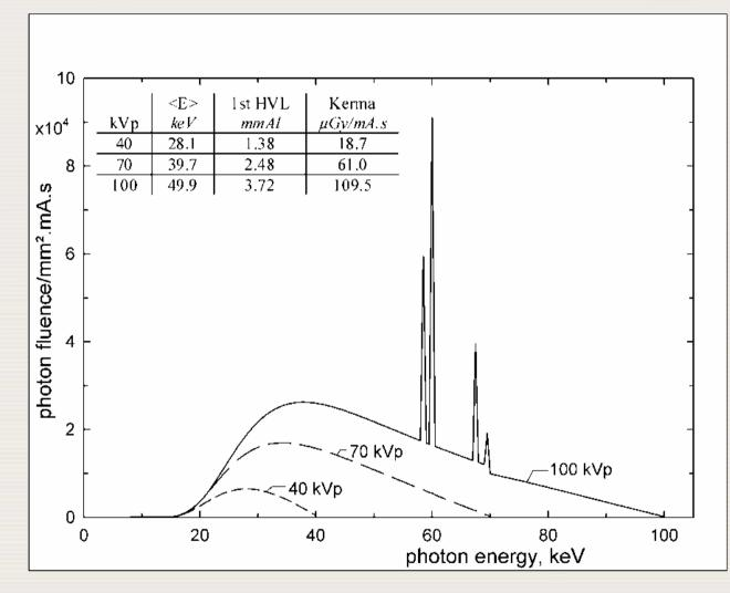
X ray spectra for various tube voltages and a tungsten target (constant voltage; anode angle 12°)
