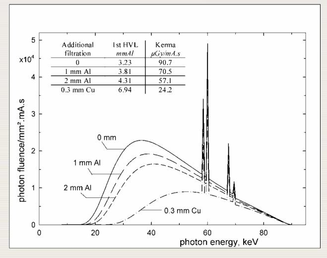
Effect of additional filtration on the X ray spectrum (90 kV, 3.4% ripple)
