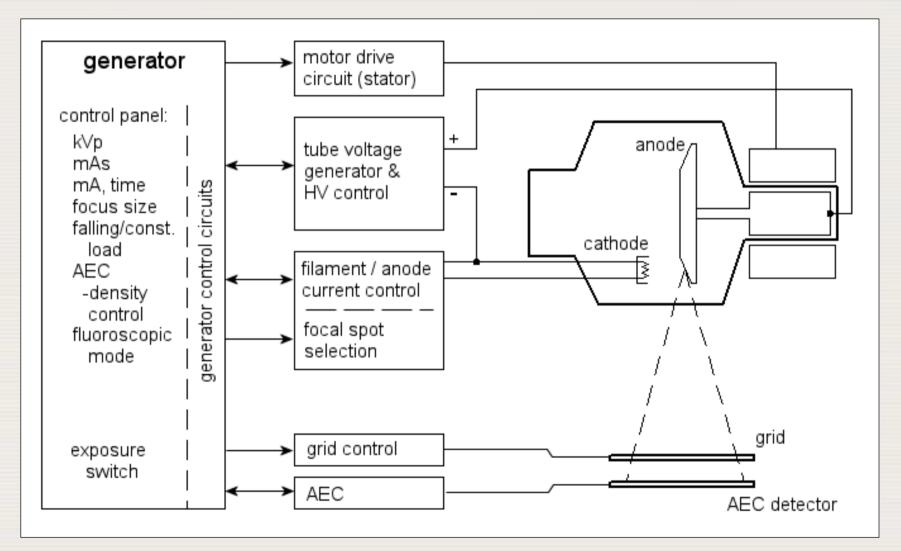
Schematic diagram of a basic X ray generator
