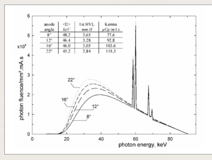
X ray spectra obtained for various anode angles and a tube voltage of 90 kV (DC)
