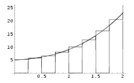
The Riemann sum corresponds to the sum of the widths times heights of the rectangles (and approximates the 'area' of the region under the curve, which represents the graph y = f(x) for  $a \le x \le b$ ). In this picture n = 8, all the widths  $\Delta x_i$  are the same and the points  $c_i$  are the middle points of the allowed interval for them.
