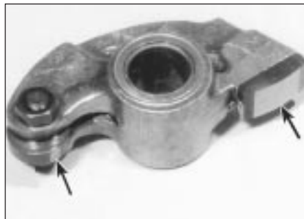
9.18 Look for signs of pitting, discoloration or excessive wear on the ends of the rocker arms where they contact the camshaft and the valve stem tip
