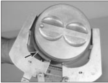
18.2 Removing the compression rings with a ring expander - note the mark (arrowed) facing up
