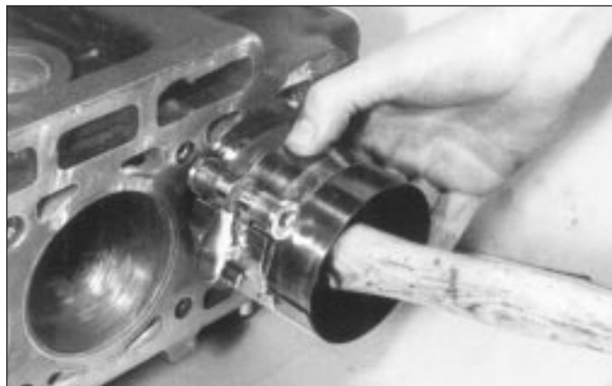
26.11 Drive the piston gently into the cylinder bore with the end of a wooden or plastic hammer handle
