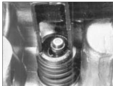
11.6 With the retainer fitted, compress the valve spring and refit the collets as shown
