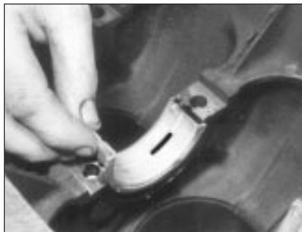
24.6 Refitting a thrust main bearing (note the flanges) in the engine block bearing saddle
