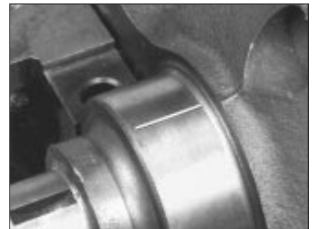
24.11 Lay the Plastigage strips on the main bearing journals, parallel to the crankshaft centreline
