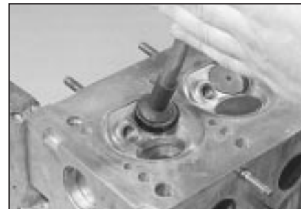
10.5 Grinding-in a valve - do not grind-in the valves any more than absolutely necessary, or their seats will be prematurely sunk into the cylinder head
