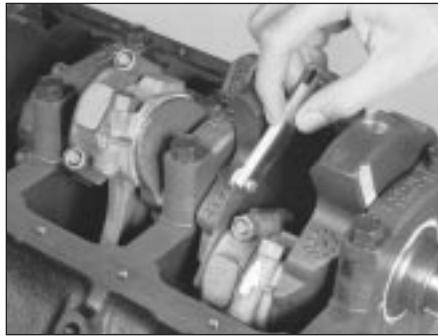
12.3 Check the connecting rod side play with a feeler gauge as shown
