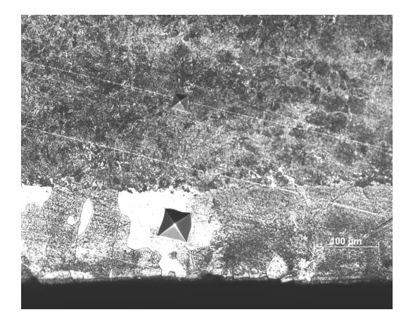
Specimen oxidized for 15 minutes at 1575F. Plane of polish is perpendicular to surface. Nital etched.
