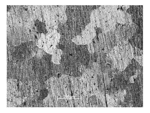
Pre-polished specimen oxidized for 15 minutes at 1575F.
