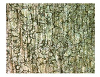
Etchant: 10% Ammonium persulfate. 6 V dc, 10 seconds.
