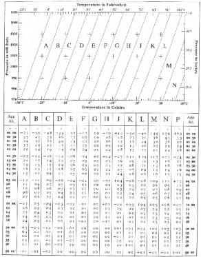
The graph is entered with arguments temperature and pressure to find a zone letter; using as arguments this zone letter and apparent altitude (sextant altitude corrected for index error and dip), a correction is taken from the table. This correction is to applied to the sextant altitude in addition to the corrections for standard conditions (for the Sun, stars and planets from page Az-A3 and for the Moon from pages xxxiv and xxxv).
