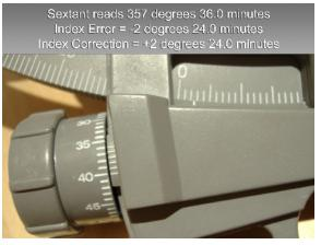
Some sextants have adjustment screws on their mirrors that can be used to 'zero' the sextant's measurement thereby removing Index Error from the equation. You should
