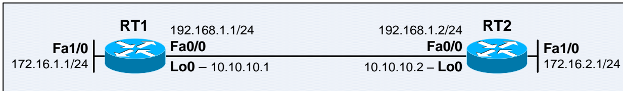
Figure A6-25: Network Setup for the show ip ospf interface EXEC Command
