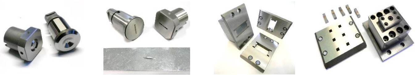
El forming UP tooling Emboss , countersink
