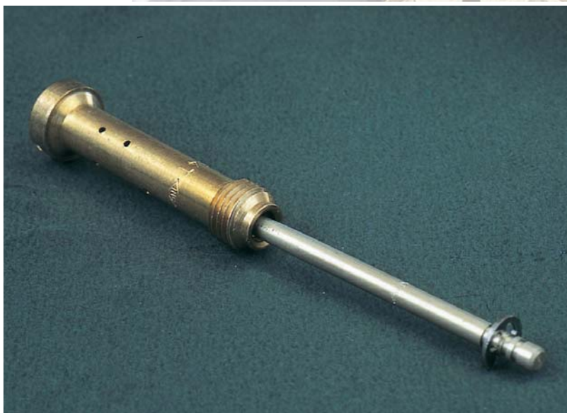
Above, the group of main and starting jets inside the float chamber. We can note the baffle that keeps fuel in the chamber of the main jet even when the motorcycle is subjected to acceleration that would tend to move the liquid mass in the float chamber. Below, the conical needle and atomizer placed in their relative working positions.
