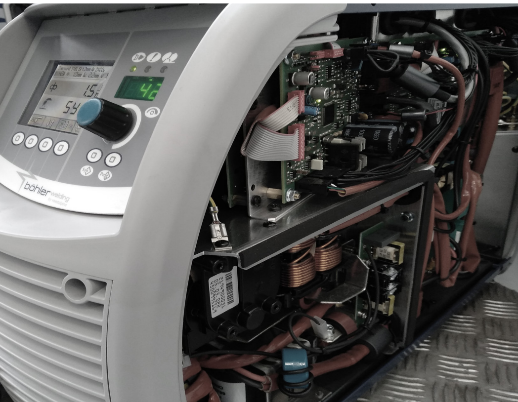
Figure 2: Design of a modern welding power source (source: voestalpine Böhler Welding)
