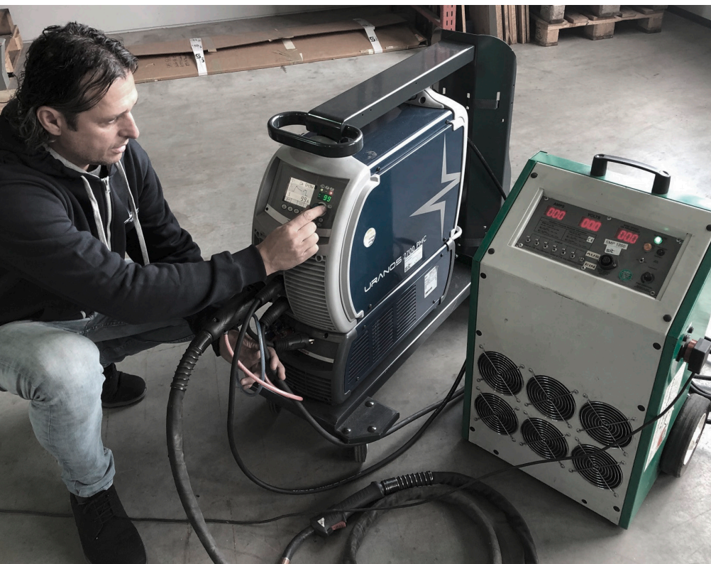
Figure 5: Calibration of a welding power source using a calibrator (source: Schweisstechnik Jantscher)
