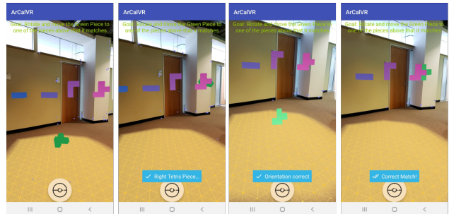
Figure 14: Tetris puzzle: the user needs to move and rotate the green puzzle piece in the AR space using taps and swipes to find and match the position and orientation of another piece.
