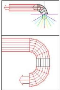
2. When you insert multiple objects CADvent controls the connections. CADvent does not allow e. g. that you connect a damper directly to a tee. Like shown in the picture on the right you cannot snap the connection point, but instead the middle point is shown. But if you mount a connector (in this example a coupling because both products have male fittings), then CADvent allows to mount the damper to the coupling of the tee.
