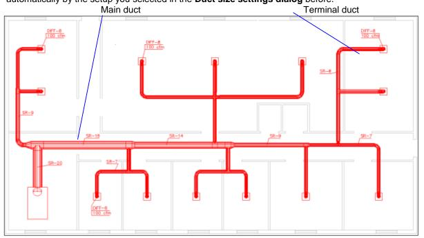
Duct system after sizing
