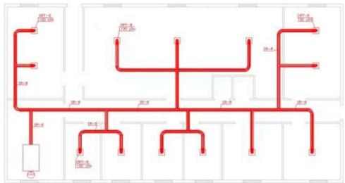
Duct system before automatic sizing
