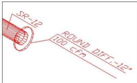
Mount a diffuser to a duct
