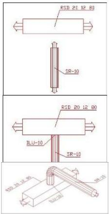
Connect round duct to rectangular duct- Method
