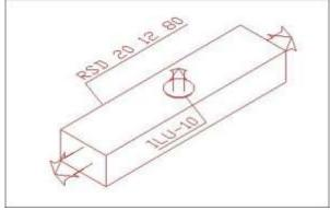
Connect round duct vertical/horizontal with a Take-off to a rectangular duct
