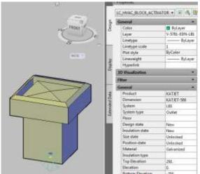
Special Terminal inserted from database into drawing
