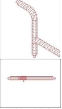
Continue vertically from a duct in plan view
