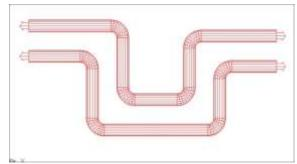
Duct system copied with "Offset Copy" command
