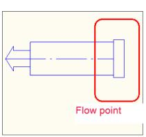
Flow Point inserted at connection point
