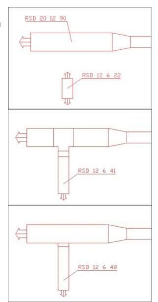
Connect two rectangular ducts with different elevations
