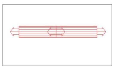
Break Duct Function - Split Duct in Two Parts
