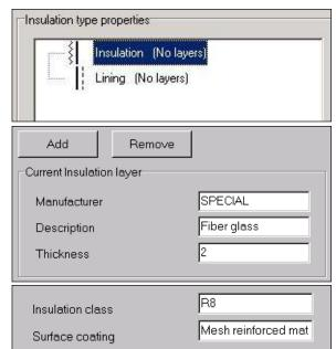
Insulation Type Properties Section of Insulation File dialog
