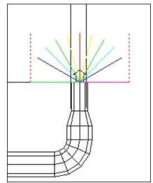
Track size command – Automatic sizing from 2D-drawings
