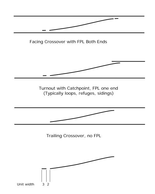
For crossovers or turnout with catchpoints, insert xover from one track to the other then insert straight line to indicate FPL
