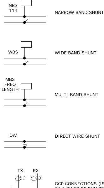
GCP CONNECTIONS (ISLANDS) (NB TX LEADS TO BE SHORT) TX & RX TO BE RUN SEPARATELY
