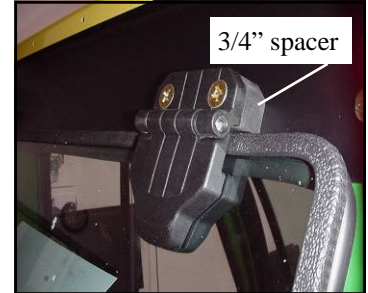
Fig. 8.2 Install Rear Window
