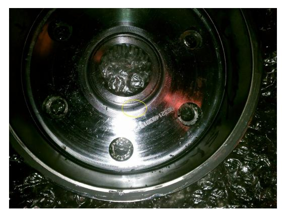
If you look carefully at the photo of the rotor above, you can see the tiny oil spraying hole in the area circled in yellow. It looks tiny, but it doesn't take a very big hole to spray enough oil to cool things down.
