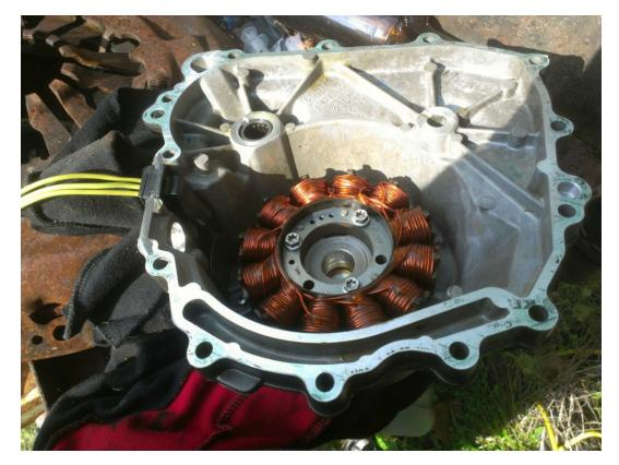
I got everything buttoned up, again, and tested it out. Note that the picture was taken with the bike under high electrical load (hot motor, fans running on high, high beams on). This is also with the CE-605 SB regulator hooked up, which works nicely with a properly working stator.
