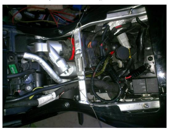
I also removed the band-aid charging "upgrade harness" from the bike. This uses a relay to turn off 2/3 of the stator to try and manage heat. This is incompatible with the CE-605 SB, and is no longer applicable with the oil spraying rotor.
