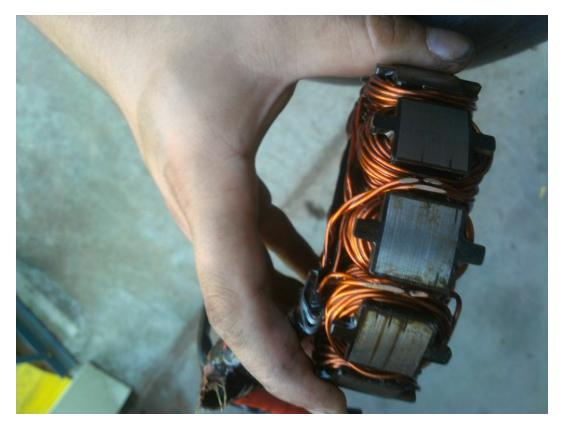
The windings were too messy, and some made contact with the rotor, and eventually rubbed through. Unfortunately, this took a toll on my new rotor as well. Rotor is still working fine, it just looks ugly. Next time I have the motor apart for a valve check/adjustment, I'm going to fill in the damaged section with epoxy.
