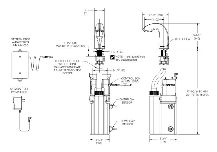
\*\* NOTE: Battery pack or AC adaptor required. AC power source required to be within 54" (1371) of the control box.
