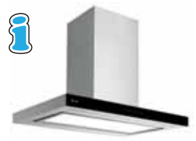
ZI922 Island hood, W900mm Illuminated touch controls Three speeds, LED lights 587m 3 /h, B energy Stainless steel and glass Recirculation kit CAP61CF Ref: 043080
