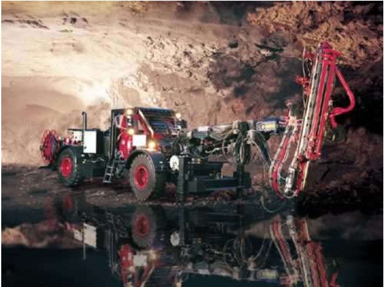
The JAMA DBU 800 underground drill/bolt machine.
