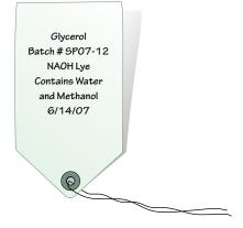
Container labels should indicate the type of fluid, any distinguishing characteristics, and the date the fluid was produced or stored. Dating waste containers is particularly important to be sure that storage does not exceed the one-year limit regulated by the PADEP. Methanol containers should be labeled "flammable" and lye or KOH containers should be labeled "corrosive." Stickers for labeling may also be available from chemical suppliers.
