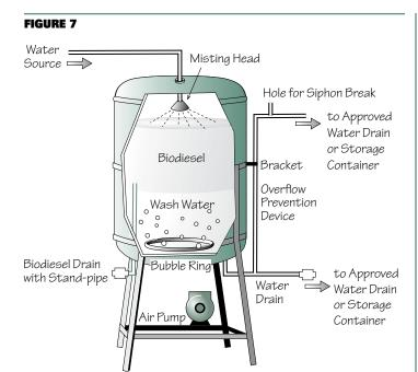
droplets onto the surface of the fuel and the water settles to the bottom of the tank drawing impurities with it) or bubble washing (air bubbles are pumped into clean water at the bottom of the wash tank, where they rise and pull the water into the fuel, gently circulating the water until it is saturated with impurities.) Bubble washing is an effective way to reduce the total amounts of water used and waste produced, since it recirculates water through the fuel several times over.
