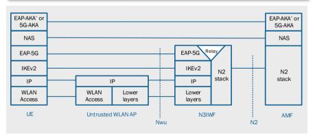
Control plane for Signaling IPsec SA for Untrusted WLAN
