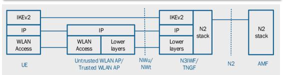
User plane for transport of data over WLAN Access
