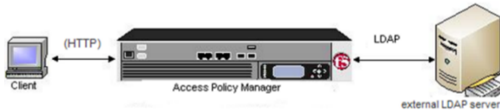
Figure 2: How LDAP works
