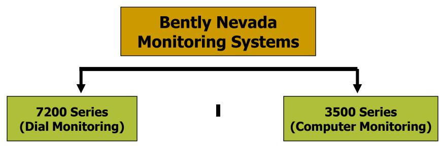
we have two types of vibration monitoring system the Bently nevada 7200 series vibration monitoring system. It is a dial monitoring analog system installed at our plant on Air Compressor partially and on Most of the TPs etc.
