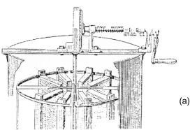
Movable frames can be spun in a radial (a) or tangential (b) extractor Both of these can be adapted to take comb from the top bar hives by making wire mesh cages that sit where the frames normally would A third option (not shown) is for flat, round mesh trays that stack inside the cylinder.
