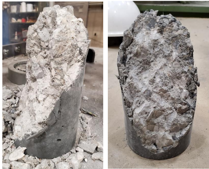
Figure 3.12. Examples of failed UHPC slant shear specimens
