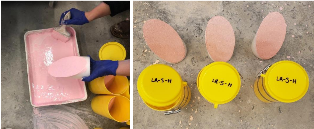
Figure 3.2. Formwork retarder application
