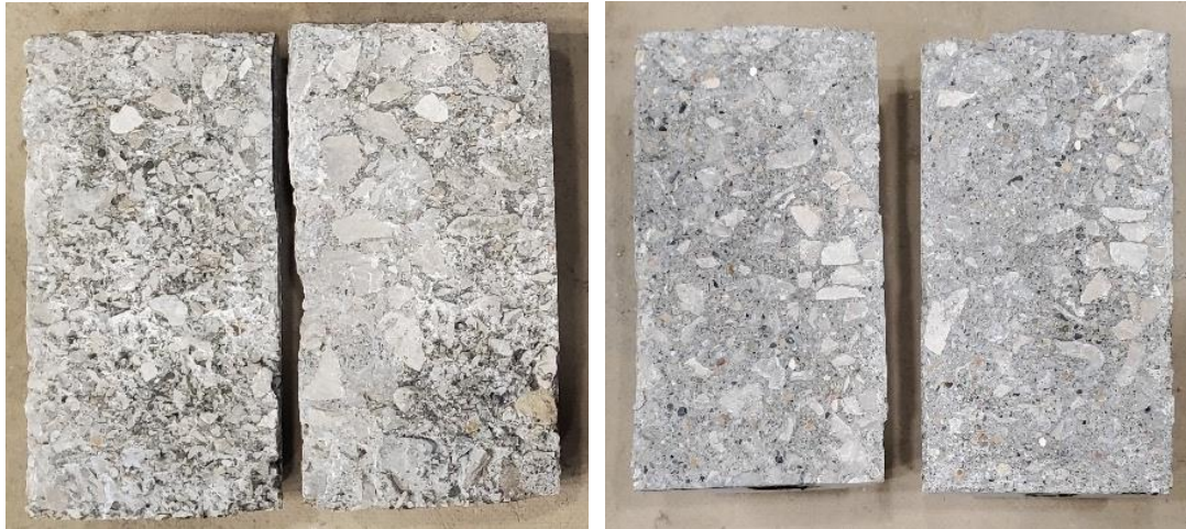
Figure 3.10. Examples of partial substrate failure: HESC (left), SCC-C (right)
