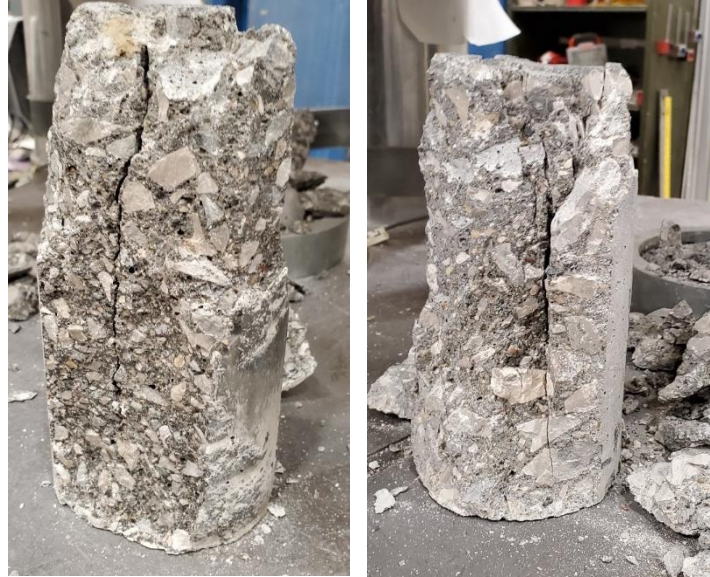
Figure 3.11. Examples of failed slant shear specimens: HESC (left) and SCC-C (right)
