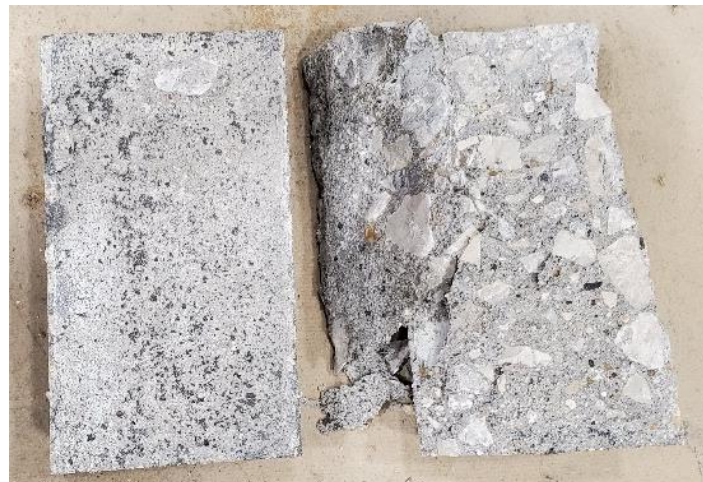
Figure 3.9. Example of UHPC-NP specimen after failure
