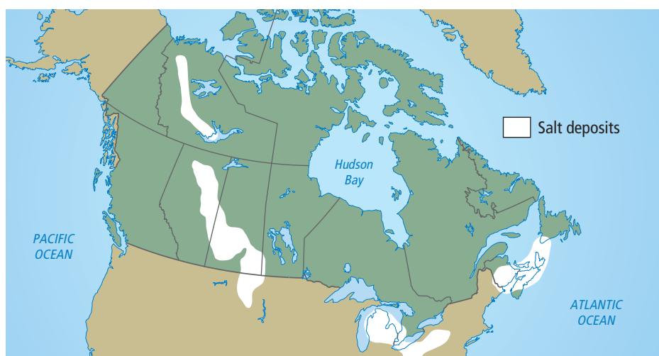
Figure 5.13 Western Canada has a huge deposit of rock salt that averages 122 m in thickness, covers approximately 390 000 km 2 , and contains more than a million billion tonnes of salt. The salt is mined for use as road salt.
