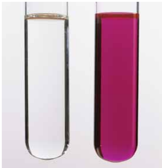
Figure 5.5 Phenolphthalein indicator in an acidic solution (left) and in a highly basic solution (right).
