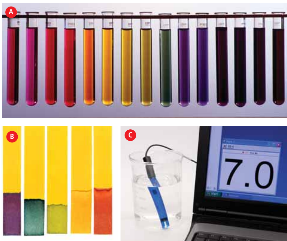
Figure 5.4 Universal indicator can be prepared as a liquid and then dropped into a test sample (A), or it can be dried onto paper called pH paper (B). The sensor is measuring the pH of a solution (C).
