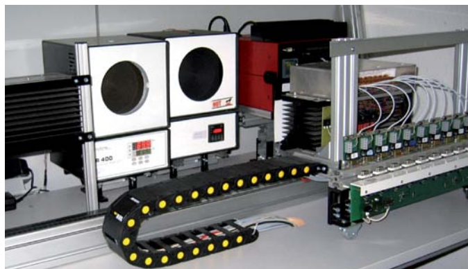
Automated calibration stations at Optris GmbH
