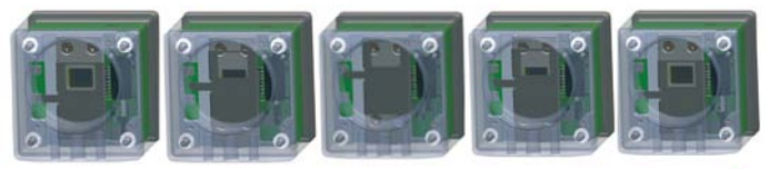
For offset compensation the whole field of view of an infrared sensor array is closed by a linear motor for a short time
