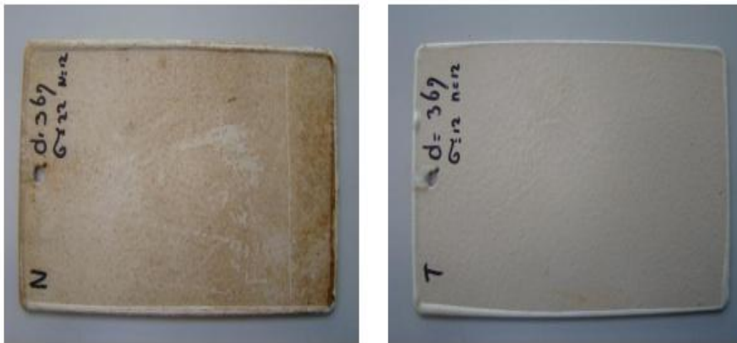
Figure 4. Intact coated panels in untreated water for 90 days (left) and intact coated steel panels in treated water for 90 days (right).
