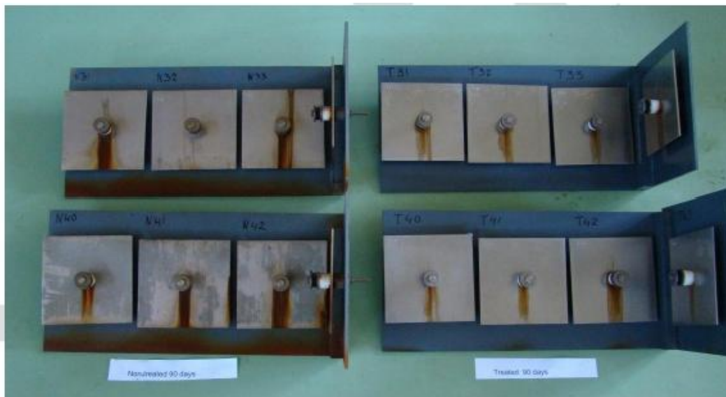
Figure 3. Corrosion on AISI 316 (top) and AISI 304L (bottom) materials in untreated seawater (left) and treated seawater from the ERMA FIRST BWTS (right) after 90 days.
