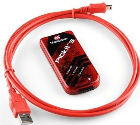
Microchip development kit: programmer software (MPLAB IPE) + hardware (PicKit3)
