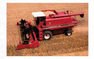
The introduction of the first 300 Axial-Flow® combines occurred in 1977 in the U.S., offering two new models, the 1440 and the 1460. The first Axial-Flow<sup>®</sup> combines featured manual hydraulics, an open centre hydraulic system (gear pump) as well as manual and automatic header height controls. This was followed by their launch in Australia in 1978-79.
