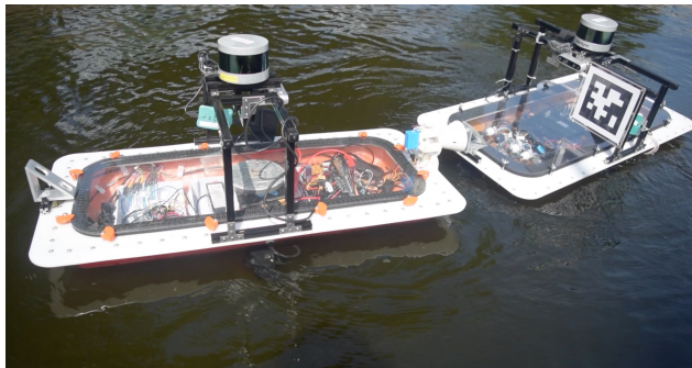
Fig. 1. Autonomous robotic boats latched in train link configuration.
