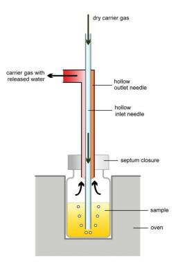
Fig. 4: Principle of the oven technique
