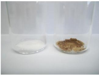
Fig. 3: Sodium tartrate dihydrate before (left) and after (right) running a temperature gradient.
