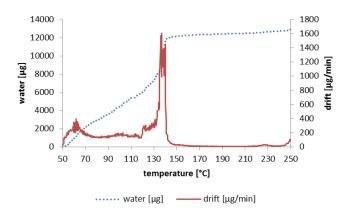
Fig. 2: Temperature gradient of sodium tartrate dihydrate showing the amount of released water and the associated drift value as a function of the temperature
