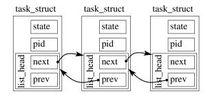
Fig. 6. Illustration of linked-list sub-object in Linux kernel
