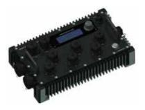
The RIS is a rugged hardware platform that hosts analogue and digital radio gateways and supports IP networking, routing and Radio over Internet Protocol (RoIP). It provides the flexibility to bridge disparate radio networks together and when used with the Currawong Battlespace Communications System it can extend the range of tactical radio nets through the network.
