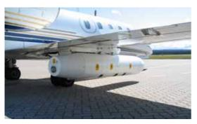
The Future Advanced Threat Simulator (FATS) is a third generation Anti-Ship Missile threat simulation product offering Navy customers the ability to trial their ASM countermeasures and overall ship preparedness in peacetime. The core FATS capability is a radar system simulating ASM threats in I, J and K frequency bands. FATS is designed to operate in Laboratory, Clifftop, Flight and HWIL configurations. Transfer between configurations is enabled via common hardware and software blocks.
