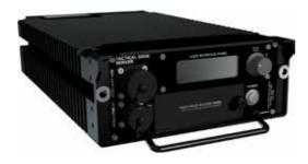
The TES is a passively cooled, ruggedised computing platform that brings server class performance and storage to the battlefield allowing de-centralised "Edge" computing. The TES uses an industry standard and upgradeable Computer on Module (COMe), with the current model providing a Gen6 Intel Xeon processor, 48GB of RAM and two configurable solid state drives for storage. Future TES models will support the latest Intel Processors.
