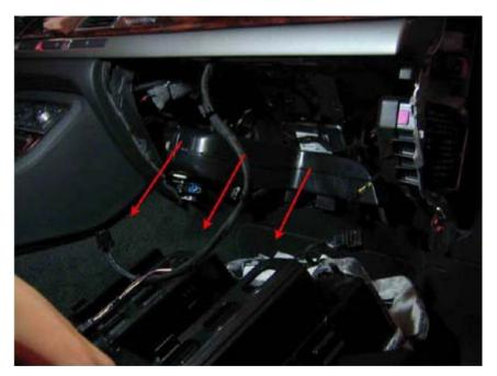
**Step 5**Unplug the original OEM Monitor Cable from the Control Box.
