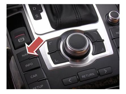
Press the Navi button and then select the required Video Source from the on-screen options.
