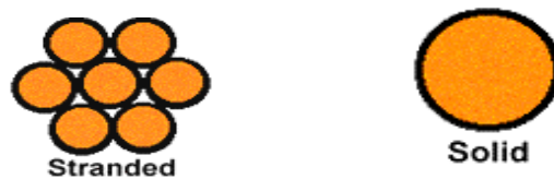
Figure 5.2 (Stranded & Solid Wire)
