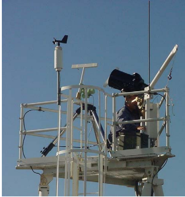
Figure 8.5 – The top of the test stand with the seeing monitor (right), weather station anemometer (left), and mobile SHABAR unit (center)
