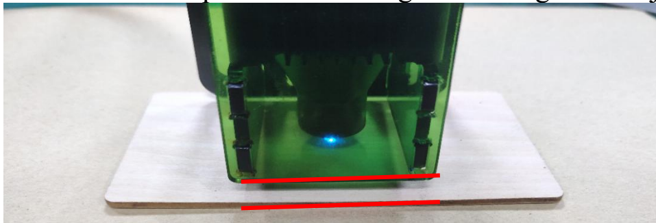
Picture 3.2 The shield is parallel to the edge of the engraved object
