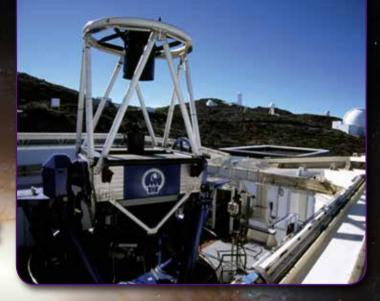
The felescope has a main mirror of 2m across and weighs 23 tonnes. The LT is sited 2,363m above sea-level on the island of La Palma in the Canaries, but is remotely controlled from the Astrophysics Research Institute. Indeed the LT is the largest fully-robotic telescope ever built. Students on our programmes have unique access to this premier international research facility to conduct research at the very frontiers of knowledge.
