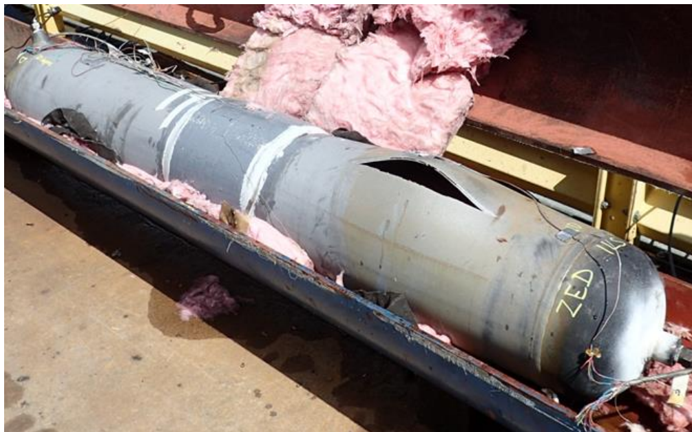
Figure 4-1: Inter-layer strain sample after burst test
