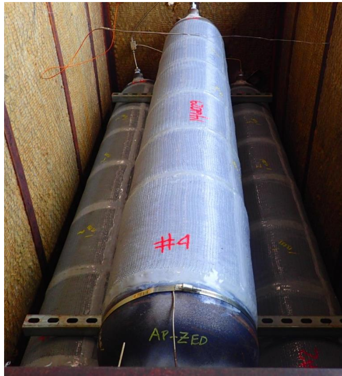
Figure 3-7: Three ZED 1,000 hour samples in insulated box
