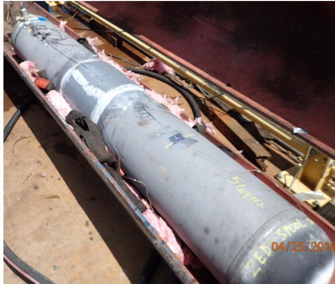
Figure 3-4: ZED spool survival sample in burst tube pre-test
