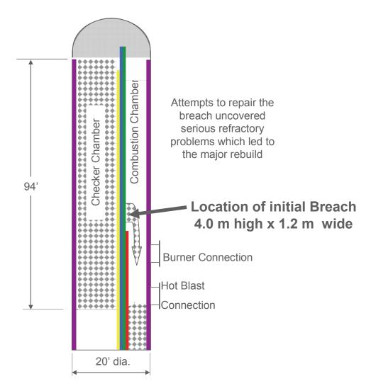
Figure 1 Stove Vertical cross-section with the damaged area
