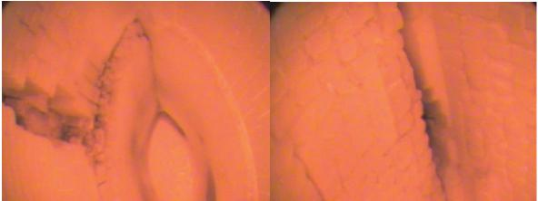
Figure 9: #6 Stove Combustion Chamber wall and corner failures
