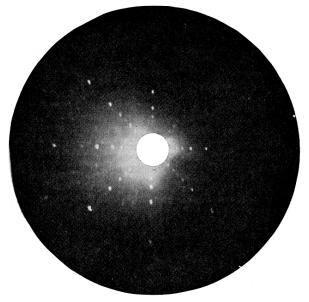
Fig. 6-7. Laue spot pattern formed by X-rays diffracted by NaCl.
